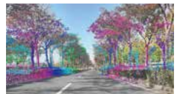
Combined LiDAR + camera calibration
